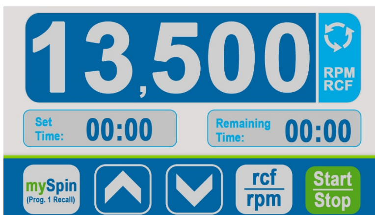
Figure 2. C0817-V control panel layout
