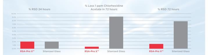
This graph displays data from our lab demonstrating the range of quantitative differences in silanized glass vials versus the RSA-Pro X<sup>™</sup> vials over 72 hours, in aqueous conditions compared to "silanized" glass vials.
