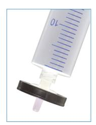
Using MicroSolv NDX™ Nylon multi-depth syringe filters allows you to filter viscous and highly particulated samples with less back pressure and therefore less hand force/stress. Made with 3 layers of varying pore size microfiber glass and one layer of low extractable nylon these filters are excellent for any hard to filter sample. Often the first choice in dissolution testing, environmental and other labs using many different complex mixtures
