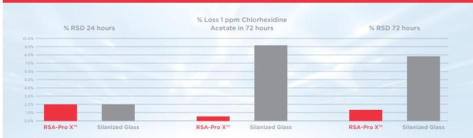
This graph displays data from our lab demonstrating the range of quantitative differences in silanized glass vials versus the RSA-Pro  $X^{\text{TM}}$  vials over 72 hours, in aqueous conditions compared to "silanized" glass vials.
