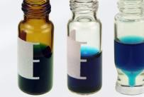
NOT ALL GLASS VIALS ARE CREATED EQUAL AND THEY ARE NOT INERT. The glass surface is covered with highly reactive silanols that can interact with your samples by changing pH, hydrolyzing or adsorbing it and lowering your quantitation results with a poor RSD.
