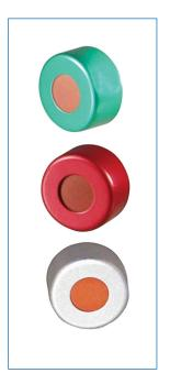
Standard, aluminum crimp caps for serum or snap-top finish 11mm, 2ml vials. Our caps are made with silicone rubber instead of natural red rubber and therefore offer better resealing, softer on the instrument and needles are cleaner; at the same cost.
