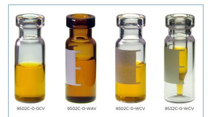
Standard crimp top style vials for HPLC or GC autosamplers. The serum finish, 11mm (ND11), allows for crimp caps to form excellent seals. The wide opening of these vials allows for easy filling and decanting and prevents "vapor lock" during filling.
