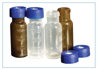
These inert, plastic vials are designed for easy sample removal and have a slightly concave inner base that helps to reduce dead volume. Offering a high volume (2ml), these plastic vials are useful when glass causes problems for chromatographic reproducibility. Compatible with almost all autosamplers that accept 12 x 32mm vials. Caps are sold separately.
