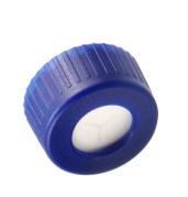
These screw caps are fitted with septa that have the highest quality silicone rubber laminated with PTFE. The silicone rubber is precut or slit into a Y shape to allow for thick or dull needles to penetrate them. The PTFE is not slit and offers protection from evaporation until the septum is pierced.
