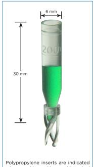
Polypropylene inserts are indicated when working with any biological compound that may adhere to glass or small molecules that might interact with or be adsorbed by the vial.
