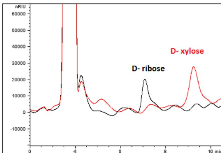
It is important to note, Refractive Index instruments are very sensitive to temperature and mobile phase fluctuations. It is very important to be aware of these factors as well as maintaining a proper calibrated machine, as goes with any instrument.
