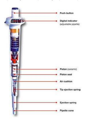
Above is a schematic of a typical pipette.
