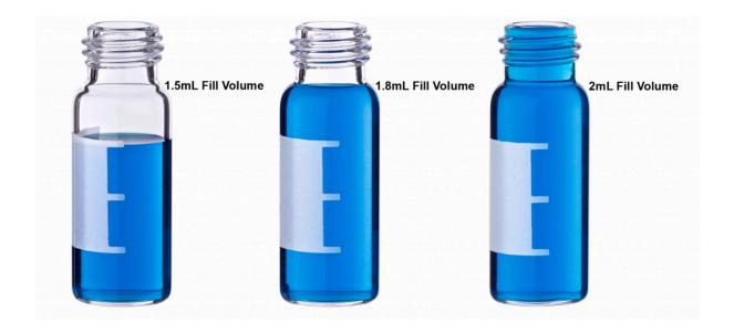
As shown above the Volume of a 12x32 mm screw vial when completely filled, it will contain approximately 2mL. This volume for Autosampler filling is called a total fill volume. When other volume designations are used, this is called a nominal volume.
