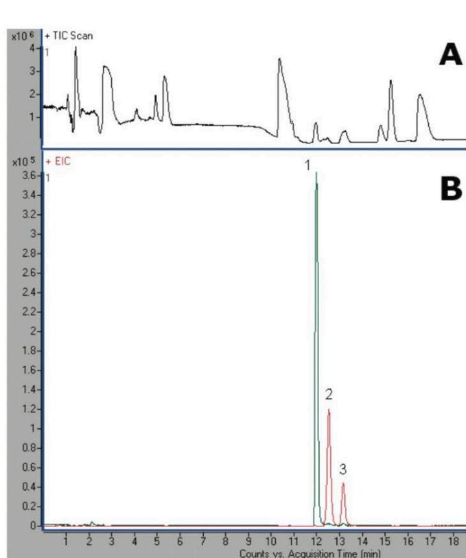
A- TIC – Total ion chromatogram of synthetic urine sample
