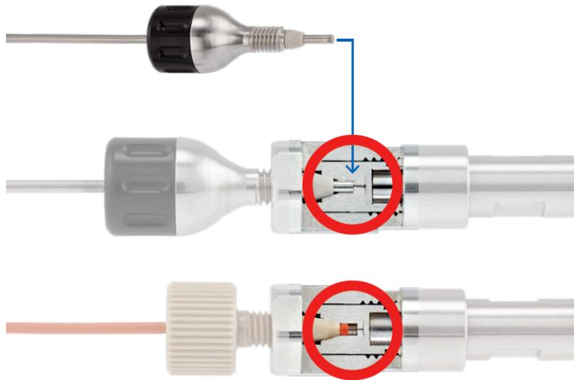
Above Circle: Spring Loaded Di-Ad Adjusts to any Pilot Length Bottom Circle: Poorly Adjusted Pilot Length
